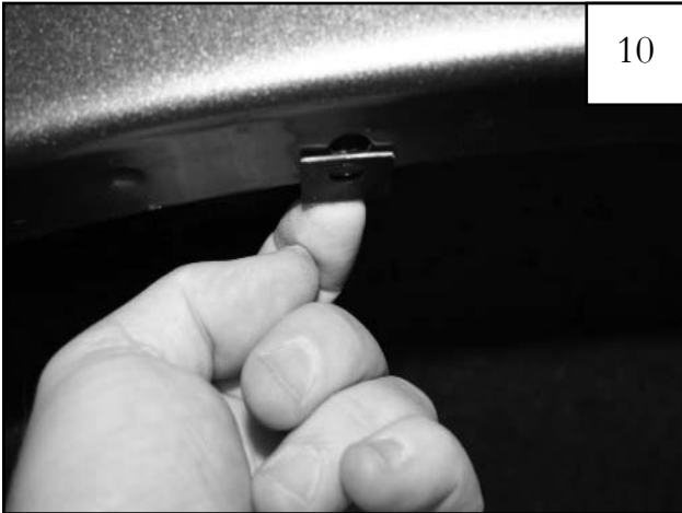
Install Clip (CL1-0022) over existing factory holes. There are two holes at the top center location. The hole for proper installation is the one toward the front of the vehicle. NOTE: The clip may fit over the lip loosely. This can be fixed by pinching the clip more tightly to the vehicle.
