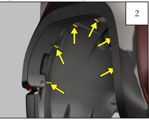
While holding the front flare in place, mark the flare's (6) hole locations using a grease pencil. (Wheel removed for visual clarity.)
