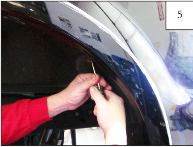
Using a pry tool, remove two factory installed tufloucs from splash guard
