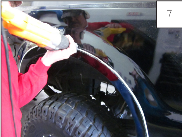
Using a sawsall, cut along inner edge of tape line. WARNING: Angle blade downward/inward for a better (angled) cut in the double walled sheel metal and to avoid cutting support rod . See next step.
