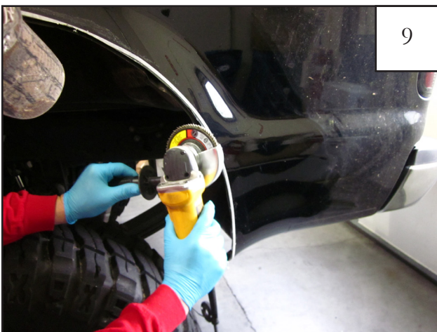
Using a grinder, deburr cut edges. Treat any bare sheet metal with rust resistant paint BEFORE continuing.
