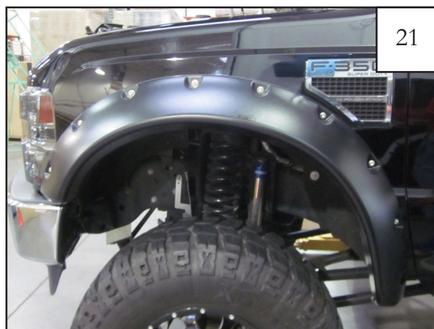
Completed front flare installation.
