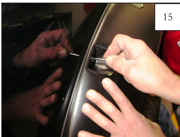
Hold flare in place. Using a scratch awl and pocket holes in flare as a guide, mark vehicle for drilling.
