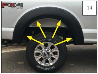
While holding flare to vehicle, start supplied screws (SW1-0058) through the four topmost mounting holes in flare and into the clips installed in Step 12.
