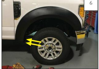
Still holding flare to fender, re-install remaining factory screws removed in Step 1 using 7mm socket and wrench. Tighten all screws.
