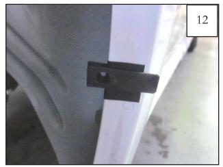
Install a Clip (CL1-0009) over each of the four Tabs (MT1-0034) placed over the upper 4 marks made in Step 10.
