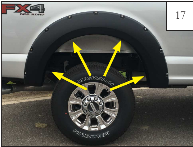
17 While holding flare to vehicle, start supplied screws (SW1-0058) through the four topmost mounting holes in flare and into the clips installed in Step 18.
