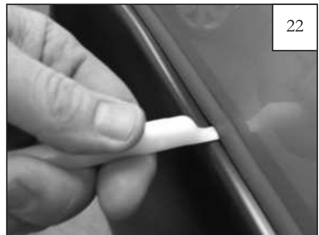
22 Using flat end of supplied Edge Trim Tool (ET1-0002), seat edge trim against flare by inserting straight end between edge trim and flare at one end. Next, slide around entire edge to the other end.
