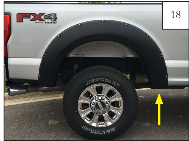
18 Start a supplied screw (SW1-0050) through the flare into the clip installed in Step 19. Tighten all screws.
