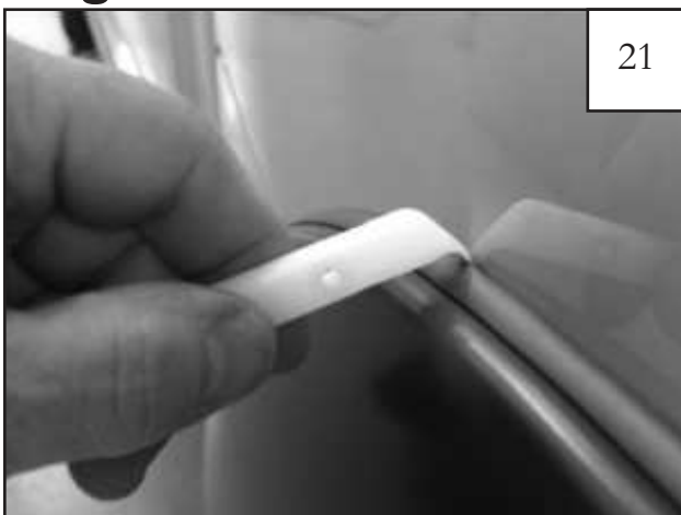
21 Using supplied Edge Trim Tool (ET1-0002), seat edge trim against vehicle by hooking curved end under edge trim at one end of flare. Next, slide around outer edge of flare to the other end.
