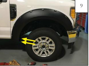
Still holding flare to fender, re-install remaining factory screws removed in Step 4 using 7mm socket and wrench. Tighten all screws.
