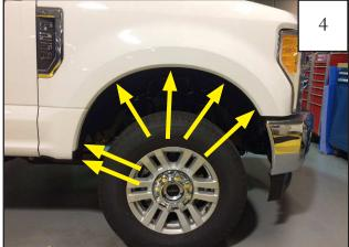
Remove six factory screws with a 7mm socket wrench. Save screws for reinstallation. **Note:** For Platinum Edition, after you remove the factory flare, there are additional screws to be removed. These screws will be used for reinstallation.
