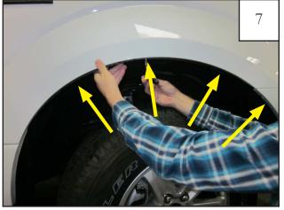
Using a 7mm socket wrench, reinstall the factory screws through the inner piece.
