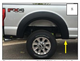
Start a supplied screw (SW1-0050) through the flare into the clip installed in Step 6. Tighten all screws.
