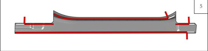
Peel back roughly 3" of red tape liner from the pieces of tape on the back side of rear part. Make sure red tape liner will be accessible when part is attached to truck.
