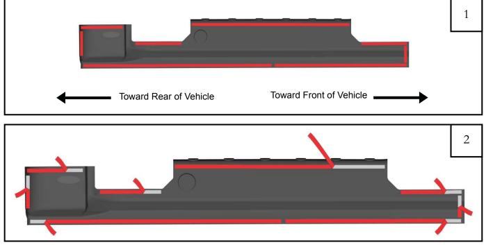
Open vehicle doors. Clean all dirt and debris from vehicle door sills and rocker panel. Use supplied alcohol wipes where part will attach.
