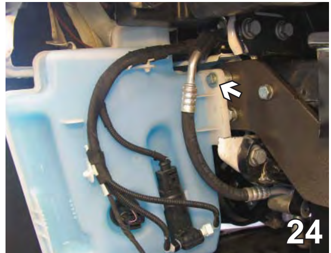
24. Using a 6MM hex bolt lock and flat washer. Install the six 3/8" lock washers between the reservoir and baseplate, then tighten water reservoir to its original location.
