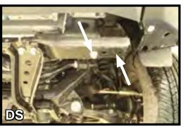
2. On 2011-2012 models only, locate the frame extension, remove the bolt using a 12MM socket and slide outer tube out. The outer tubes will not be reinstalled.
