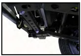
10. Align the electrical bracket with the center of baseplate cross tube, install the self tapping screws into the bottom of cross tube with the 5/16" nut driver and drill. Reposition tabs to their original placement and reinstall push pins.
