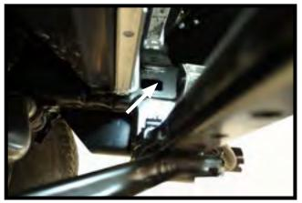
9. Remove the cap on BOTH sides of the vehicle and insert item #2, 3/8"-16 Nut Plate Weldment. Replace cap.
