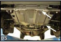
1. Using a 12MM socket remove the four (4) bolts, two (2) per side, from the belly pan and set aside for reinstalling after baseplate installation. *NOTE:* Some models may not have a belly pan.
