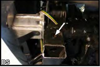
5. Insert the 7/8" O.D. spacer tube (item #9) into the opening in the side of the lower extension below the frame end so it is flush.
