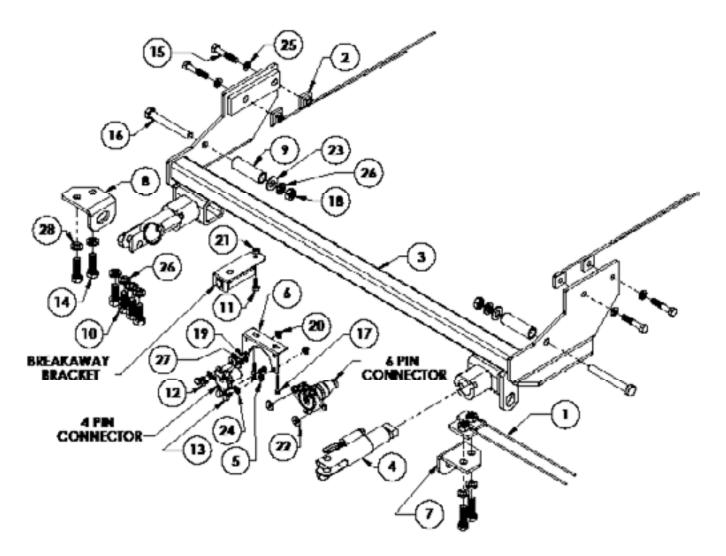
NOTE: Items #7 and #8 need to be rotated 180° for 2011-2012 models so the holes face inward. Remove existing tie down brackets prior to installing the convenience links that have been supplied with your baseplate.
