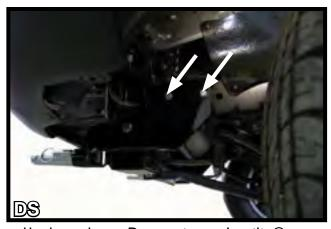
8. Align endplate with drilled holes and insert bolts and lock washers. Be sure to use Loctite® Red on all bolts prior to tightening. Replace wheel well liner to the original position and reinstall the two (2) push pins.
