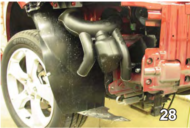
28. Reattach air baffle with existing holes and existing bolts.
