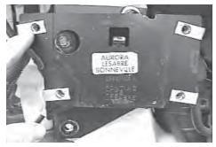
8. Remove the four clips from each bracket. They will not be used in baseplate installation.
