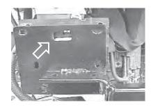
11. Set the baseplate on the hooks of the brackets. Insert both of the top bolts through the baseplate and bracket. Use appropriate hardware on bolt and hand tighten. Do the same for the other side.
