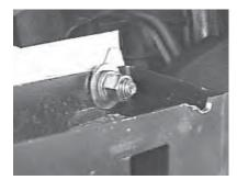
10. Drill a 3/8" hole through the bumper bracket and the frame, use 3/8" hardware as shown in drawing on page 3.
