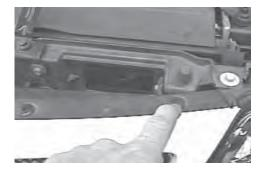
1. Lift hood and remove push pins holding top of the bumper facia.
