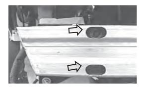
6. Remove the bolts from the bumper exposed by the slots on each side.
