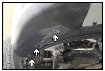
4. On the underside of the fascia, remove the three (3) push pins in the outer edge. Do this on both sides of the vehicle.
