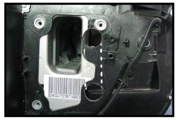
Using a 1-1/4" holesaw, drill out the two (2) holes. Using a reciprocating saw, connect the two (2) holes. Do this on both sides of the vehicle.
