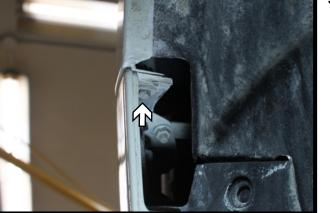
3. Using a 7MM socket, remove the screw from the top edge of the fascia in the wheel well. Do this on both sides of the vehicle.
