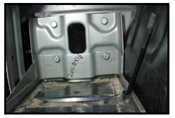
19. On the driver side, remove the four (4) 8MM bolts from the baseplate. Reinstall the battery tray with the 8MM bolts and the 8MM lock washers provided with loctite. Reinstall the battery and terminal connections.
