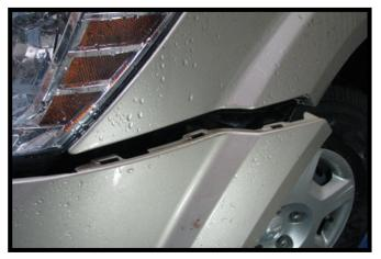
6. Lift up and pull out on the corners of the fascia to unhook it from the body. Unhook any electrical connections and set fascia aside.
