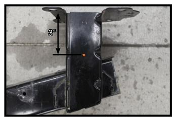
On the top side of the bumper, place a mark 3" from the back and centered across. Drill out using a 1-1/4" holesaw. Do this on both sides of the bumper.
