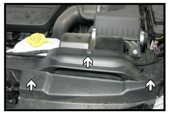
1. Remove the five (5) push pins from the top of the fascia. Three (3) on the driver side and two (2) on the passenger side.
