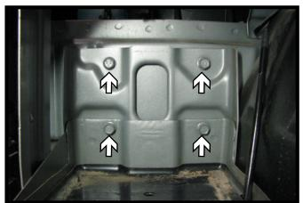
9. Using a 13MM socket, remove the four (4) bolts from the battery tray. Set the battery tray aside, the bolts will not be reused.
