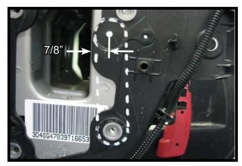
Measure from the inside of the frame over 7/8", then using the 1-1/4" holesaw bit trace the diameter. On the lower bumper bolt hole also trace the diameter of the holesaw bit. Connect the outside edges.
