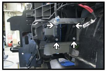
15. Slide the baseplate onto the vehicle. On the driver side, install four (4) 8MM-1.25 x 35MM bolts into the existing holes. Tighten down the bolts but DO NOT use loctite on threads at this time.
