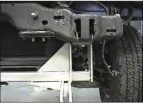
Install Base Plate according to assembly drawing on last page. Be sure and use Loctite on all bolts before tightening. Tighten all bolts according to torque chart in the General Instruction sheet.
