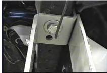
3. Align Base Plate front holes with existing holes on bottom side of frame ends. Using items 2, 4, and 5 to hold Base Plate into position, mark back holes with transfer punch. Remove Base Plate and drill hole on each side using 17/32 inch bit.
