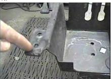
5. Hold belly pan in place, mark and trim to fit, (Refer to photo to the right), then replace bumper and belly pan. Be sure all electrical fixtures are connected and tighten all bolt according to manufacter recommendations Baseplate installation is complete.
