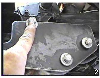
2. Hold the baseplate into place and insert the three (3) existing bolts on the driver's side through the baseplate, frame, gear box, and tighten.
