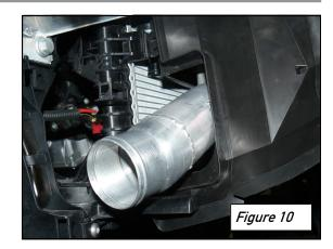
Connect the factory intercooler inlet and outlet hoses and reinstall all the bumper support factory fasteners and clips.
