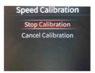
If speed sender/sensor is functioning, and your calibration successful, you may now scroll up to Back, and press Enter, then on the Speedometer Menu, scroll up to Back, press Enter, then on the Main Menu, scroll up to Close and press Enter.
