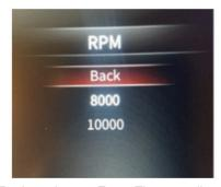
Once you have chosen the Tachometer Scaling, simply scroll up to Back, and press Enter. Then, scroll to the top until Back and press Enter. Next, once you are back into the Main Menu, scroll up to Close and press Enter.
