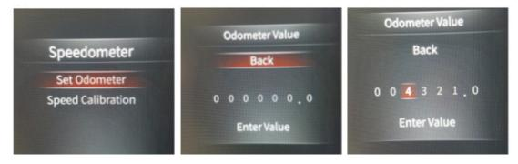
Once you have the odometer reading you desire, and have pushed Enter on the last digit, you can then scroll down to Enter Value and press Enter. The Dash will ask you "Are you sure?". You have the option to either press enter on OK, or scroll to Cancel and select Enter. This window asking you "Are you Sure?" will pop up 3 times. If you answer OK all three times, the odometer is now permanently set, and will only change by accumulating miles normally. This can not be changed again.
