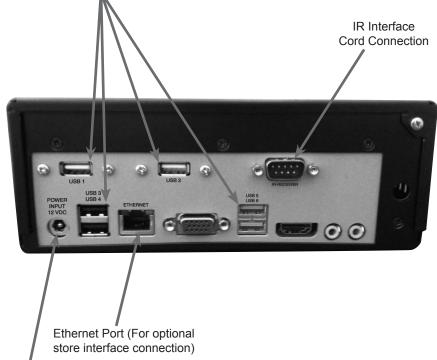
Power Supply Connection 12VDC
