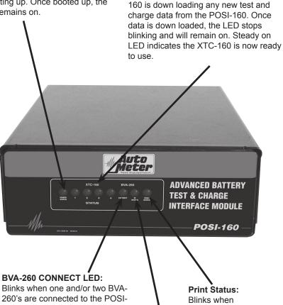
Blinks when one and/or two BVA-260's are connected to the POSI-160. BVA-260 power can be turned off. While the LED is blinking, the POSI-160 is down loading any new test data. Steady on LED indicates the BVA-260 is now ready to use.
