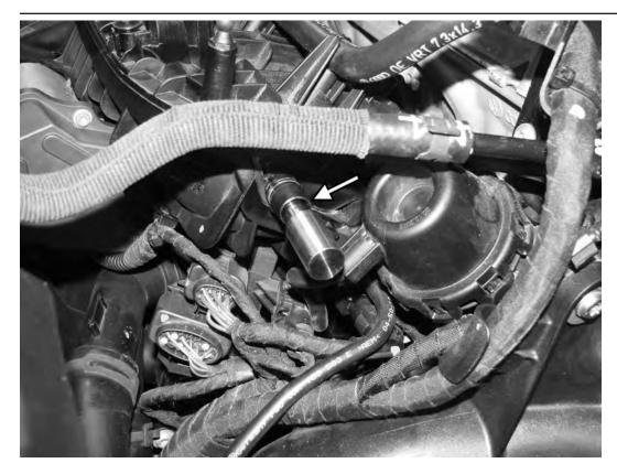
5) Locate the unused port on the front left side of the intake manifold. Place the APR punching tool loosely into this port.
