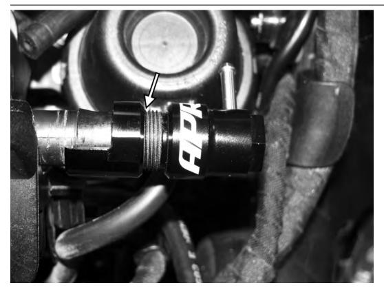
9) Begin to thread the main body of the APR boost tap into the base of the boost tap.
