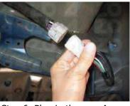
Step 6: Plug in the new Anzo wire harness into the original socket of the vehicle.
