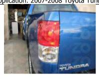
Step 1: Use the t27 torque bit socket to remove the two screws holding in the tail light.
