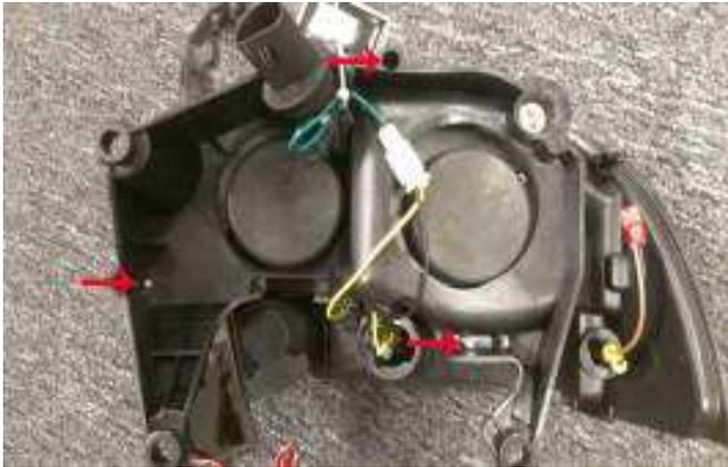
On the back side of the light there are 3 adjustment screws. You can turn these screws to move the bracket closer to the housing. by doing this you will be able to adjust the gap between the fenders and the light. You may have to take the light out a couple times and adjust the screws to get the desired gap.
