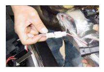
Step 8: Connect the resister pack to the headlight halo.
