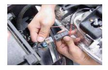
Step 7: Connect the headlight plugs into the new headlight.
