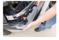
Step 4: take off the turn signals so we can splice the wires to the turn signals and halo resistor.
