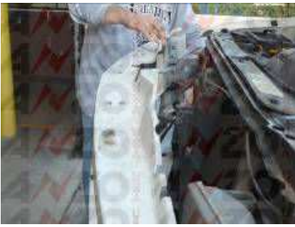
Step 8: Pull the grill away from the vehicle.
