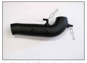
6. Install the provided 90° and straight vent fittings into the AIRAID® intake tube as shown.
