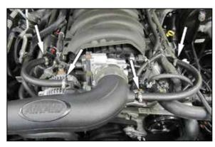
11. Install the crank case vent hose assemblies onto the vent fittings installed into the AIRAID® intake tube and then connect the quick connect fittings to the port on the valve covers.
