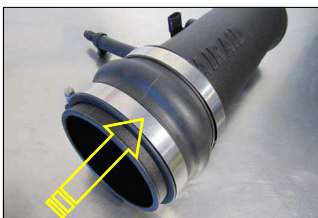
17. Slide the Hump Hose with the two 68 Clamps all the way onto the Intake tube as shown.
