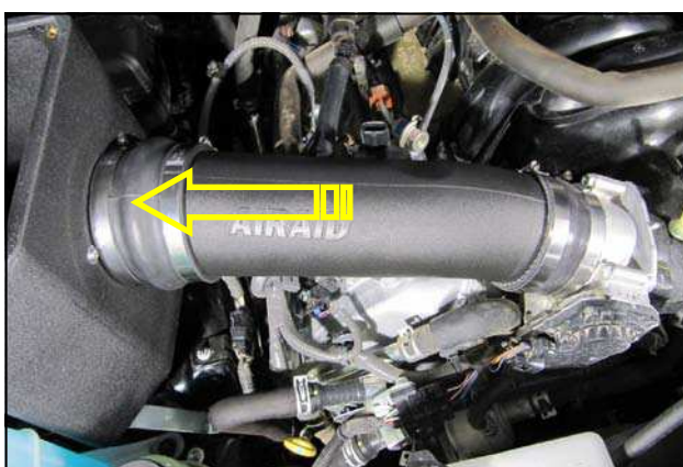
20. Slide the Hump Hose and Clamps onto the Filter adapter and tighten all four Intake Clamps.
