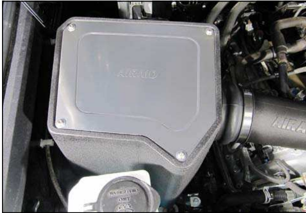
25. Remove the protective film from the other side of the Lid and mount it to the Airbox using 4 sets of 1/4-20 Button Heads, Lock Washers and Flat Washers.
