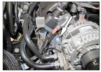
2. On vehicles equipped with a intake plenum support brace secured to the passenger side cylinder head, remove the bolt shown securing the support bracket.
