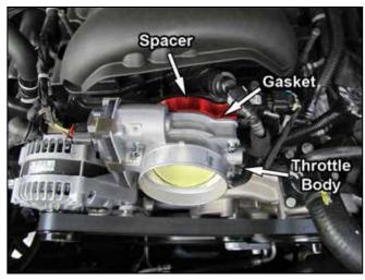
5. Install the provided new bolts through the holes in the throttle body, through the holes in the provided gasket and through the POWERAID spacer. Start the new bolts into the inserts in the intake manifold being careful not to cross thread the bolts. Tighten the bolts in a cross pattern to the factory specifications. NOTE: Be sure to install the spacer in the correct direction as noted on the spacer.
