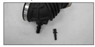
15. Move vent line fitting from stock intake tube.
