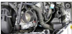
17. Install AEM® coupler on the throttle body as
