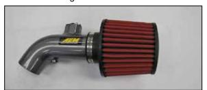
11. Install AEM® Dry Flow filter onto AEM® intake
