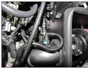
19. Install the supplied guick connect fitting onto NPT fitting, then reconnect crank case and vent line hose to the AEM® intake tube.
