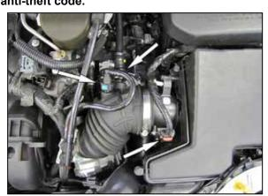
2. Disconnect MAF sensor, vent line, and crank case line from stock intake tube.
