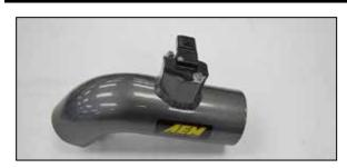
9. Remove the MAF sensor from the factory housing and install the sensor into the AEM® intake tube.
