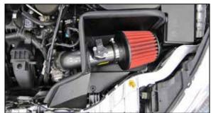
Install the AEM<sup>®</sup> intake system in the vehicle.
