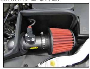
20. Route the MAF sensor wire harness through the heat shield cut out, then reconnect MAF sensor.
