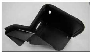
14. Install edge trim onto heat shield as shown. NOTE: Some trimming may be necessary.
