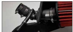
16. Install AEM® intake tube onto heat shield, then install NPT fitting and assemble the hose and quick connect fitting as shown.
