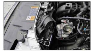
6. Pull on rubber intake duct to remove from vehicle.
