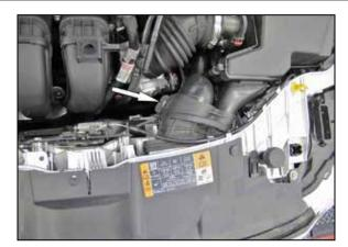
3. Release rubber strap for intake duct.
