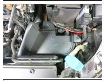
d. Install the AEM heat shield onto the factory air box mounting studs. Soapy water may be used to help the grommets engage with the studs.
