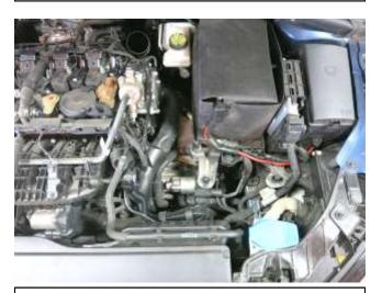
d. Remove the stock air box and intake hose assembly from the vehicle by pulling upwards to disengage the three rubber grommets. Lift the hose side first and maneuver the box towards the rear, clearing the cold air inlet.
