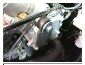
c. Install the provided rubber mount onto the side of the engine. Loosely install the provided washer and nut onto the tuber mount.
