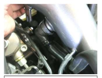
e. Position the AEM intake tube in the engine bay and connect the small vacuum hose to the small nipple. Move the large air injection hose behind the AEM heat shield and connect it to the AEM intake tube. Soapy water should be used to help installation. Note: Not all models have this large hose. Install the included blind plug (8-215) in its place.
