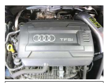
h. Reinstall the plastic engine cover by lining up the grommets with the posts and pressing down gently.
