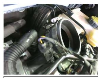
b. Install the provided coupler and hose clamps onto the turbo with the small end towards the turbo inlet. Tighten the turbo-side hose clamp to 30in-lb at this time.
