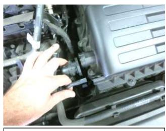
c. Remove small vacuum line from the stock air box. Remove the large air injection hose by depressing the ribbed parts of the collar. Note: Not all models will have this large hose.
