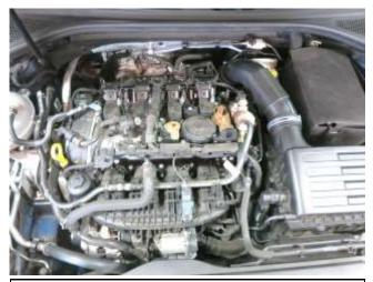
a. Remove the plastic engine cover by pulling up gently, releasing it from the rubber grommets.
