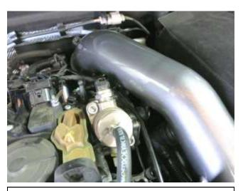
f. Lower the AEM intake tube bracket onto the rubber mount, between the washer and rubber mount, and insert the tube into the coupler. Do not tighten the mount or coupler at this time.
