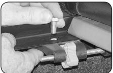
B. Slide left tension adjuster over until it engages under side rail. (See photo in Step 4 E for tension adjuster tab under side rail.) Push bar back and forth to line up holes-do not turn dial wheel. Insert bolt from top, flat washer and nut from bottom.
