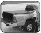
Now along side of box, seal cover edges with hook and loop scaling system the full length of cover on both sides. Pull with one hand - seal with other hand.
