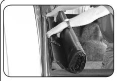
A. Set rolled up cover on rails at front of box (behind cab) with bar facing up. Roll cover bar onto front of rails and fold/tuck vinyl flap under. Now bar will face down. Let straps hang to inside of box. Push cover bar forward until it sets flat on front of side rails and overhangs them.
