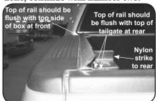
A. Position side rail with weather strip against inside lip of box. **Push rail forward until it touches front of box** (end of rail with strike goes to rear). At front, rail should be flush with top side of box. At rear rail should be flush with top of tailgate.
