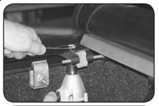
C. Hold bolt at top and tighten nut under side rail. Repeat procedure for right hand tension adjuster.
