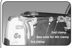
C. Install 2nd clamp on rail at midway point of box. Check if rail is level. If rail tilts up, loosen clamp, lower it and tighten. If rail tilts down, loosen clamp, raise it and tighten. Install 3rd clamp as close to tailgate as possible.
