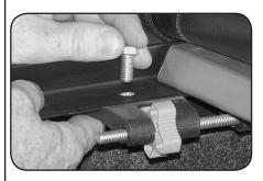
B. Slide left tension adjuster over until it engages under side rail. (See photo in Step 4 E for tension adjuster tab under side rail.) Push bar back and forth to line up holes-do not turn dial wheel. Insert bolt from top, flat washer and nut from bottom.
