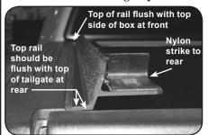
A. Position side rail with weather strip against inside lip of box. **Push forward until it touches front of box** (end of rail with strike goes to rear). at front, rail should be flush with to side of box. At rear, rail should be flush with top of tailgate.
