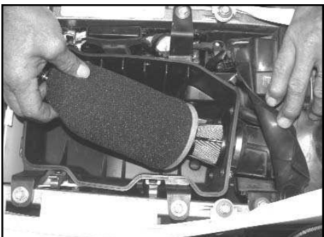
6. Remove the stock wing bolt then remove the stock air filter.
