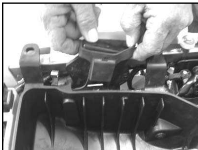
10. Remove the Engine Control Unit Assembly band.
