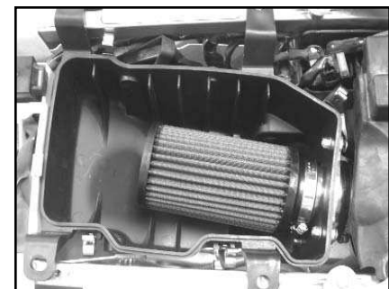
20. Install the K&N Filtercharger® onto the adapter. Securely tighten the clamp.
