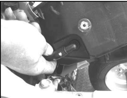
11. Lift the air box and unplug the crankcase breather tube from the side of the air box.
