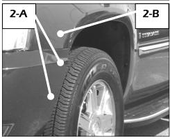
Remove the 7mm bolts and plastic fasteners attaching the inner plastic wheel wells to the bumper cover [2-A].
