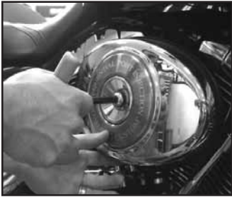
1. Remove the air cleaner cover.
