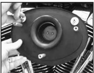
5. Remove the two stock breather bolts.
