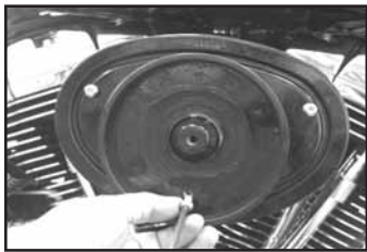
2. Remove the three button socket bolts on the K&N® air filter.
