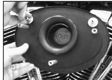
12. Reinstall the back plate and thread the stock breather bolts into the breather bolt extensions. Do not tighten at this time. Note: For 2006-2007 fuel injected models, reinstall a washer in between the back plate and each of the provided breather bolt extensions. Thread the stock breather bolts into the breather bolt extensions. There should be a washer on each side of the provided breather bolt.
