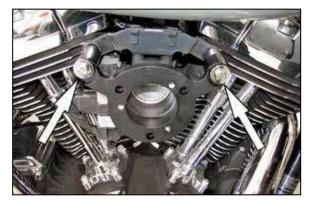
6. Install the K&N<sup>®</sup> adapter onto the engine and throttle body using the provided breather bolt. **NOTE:** Do not completely tighten the breather bolts at this time. Take care while installing the adapter so that the "O" rings do not get pinched.
