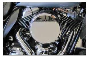
13. Install the K&N<sup>®</sup> air filter and front plate onto the back plate and secure with the provided hardware. **NOTE:** It may be helpful to use a small screwdriver to position the filter into the grooves of the front and back plate while tightening the hardware.
