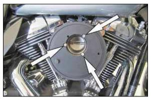
11. Install the filter back plate and gasket onto the adapter and secure with the provided bolts.
