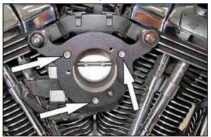
8. Install the provided throttle body gasket and then install the throttle body bolts. Secure the adapter with the two breather bolts and three throttle body bolts.
