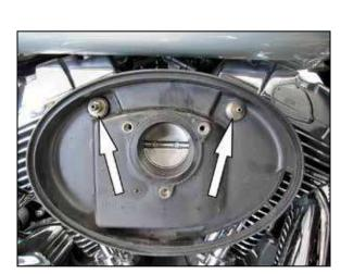
4. Remove the two breather bolts and then remove the inner air filter base.
