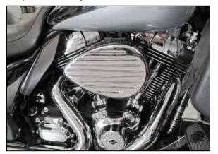
15. Install the K&N<sup>®</sup> air filter and front plate onto the back plate and secure with the provided hardware. NOTE: It may be helpful to use a small screwdriver to position the filter into the grooves of the front and back plate while tightening the hardware.
