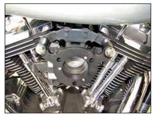
6. Install the K&N® adapter onto the engine and throttle body using the provided breather bolt. NOTE: Do not completely tighten the breather bolts at this time. Take care while installing
