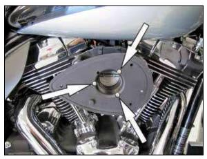
13. Install the filter back plate and gasket onto the adapter and secure with the provided bolts.
