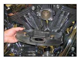
5. Remove the air filter base from the throttle body and unhook the wiring pig tail from the filter base. NOTE: K&N Engineering, Inc., recommends that customers do not discard the factory air intake components.
