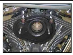
10. Install the K&N® filter base plate onto the throttle body using the factory breather bolts and the throttle bolts installed during step #7. Alternate the tightening sequence between all five bolts until the base plate is completely tight.
