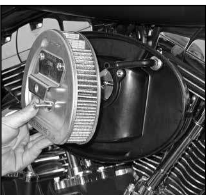
3. Remove the stock air filter element and the stock breather hoses.
