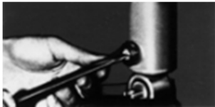
Figure 2: Turn screw from left to right to increase compression forces (clockwise) Compression - Insert a screwdriver into the lower adjustment device (figure 2). Turning the screw driver from left to right (clockwise) will cause the forces to increase. From the minimum or factory positions, there are 12 possible "clicks" of adjustment.
