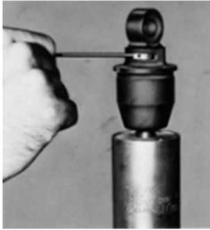
Figure 1: Move pin left or right to increase rebound forces (counter-clockwise) Rebound - Insert a pin into the slotted adjuster located at the top eye (figure 1). Moving the pin from left to right (counterclockwise) will cause the forces to increase. From the minimum or factory positions, there are 12 possible sweeps of adjustment ( 1 sweep equals 1/4 turn).
