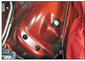
15. Install the provided rubber mounted stud onto the inner fender in the air box mounting location as shown.
