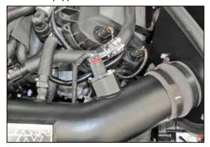
24. Connect the mass air sensor electrical connection.
