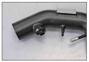
21. Install the mass air sensor into the K&N $^{\odot}$  intake tube and secure with the provided hardware.
