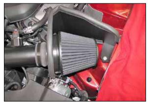
27. Install the K&N<sup>®</sup> air filter and secure with the provided hose clamp.
