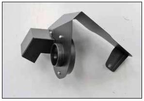
13. Install the filter adapter into the heat shield and secure with the provided hardware.
