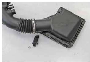
20. Remove the two screws securing the mass air sensor into the upper air box and then remove the
