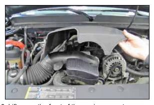
3. Lift up on the front of the engine cover to disengage from the mounting grommets. Then pull forward and remove the engine cover from the engine as shown.
