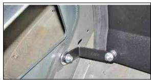
17. Secure the heat shield mounting bracket to the inner fender with the two fender washers and hardware as shown.
