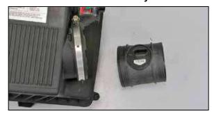
8. Loosen the hose clamp and remove the mass air sensor from the air cleaner as shown.
