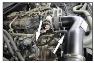
25. Install the provided crank case vent hose onto the valve cover and then onto the K&N<sup>®</sup> intake tube as shown.
