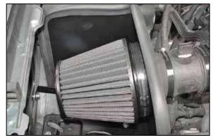
26. Install the K&N® filter as shown and secure with the provided hose clamp.
