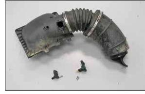
12. Remove the screws securing the mass air sensor and temperature sensor to the air box and then remove the mass air sensor and temperature sensor from the air box.
