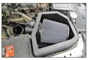
15. Install the K&N<sup>®</sup> mass air housing onto the mounting studs and into the K&N<sup>®</sup> air filter. Secure the housing to the studs with the provided hardware and then secure the air filter with the hose clamp provided.
