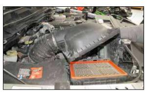
4. Release the two clips securing the air box lid and then remove the air box lid and intake tube from the vehicle.
