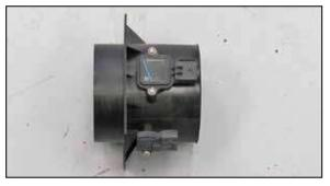
13. Install the mass air sensor and map sensor into the K&N<sup>®</sup> mass air sensor housing using a twisting motion to aid installation and then secure with the provided hardware.
