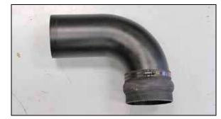
16. Install the provided silicone hose (08695) and hose clamps onto the K&N<sup>®</sup> intake tube as shown. **NOTE: Do not completely tighten at this time.**
