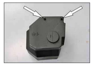
10. Install the two provided air box mounts to the bottom of the air box and secure with the provided hardware.
