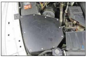
18. Install the air box lid and secure with the provided hardware.
