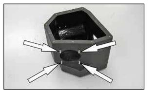
9. Install four of the provided 6mm studs into the K&N<sup>®</sup> air box as shown. NOTE: Install the studs so the shorter threads are threaded into the air box inserts.
