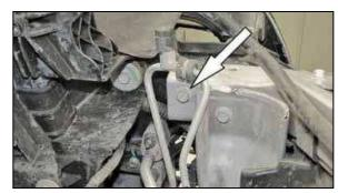
7. Remove the core support bolt shown. **NOTE: This bolt will be reused in the next step.**
