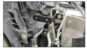
2. Disconnect the Mass air sensor and temperature sensor electrical connections, and then unhook the wiring harness from the air box.
