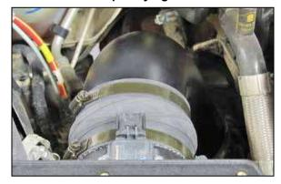
17. Install the K&N<sup>®</sup> intake tube into the factory turbo inlet hose and then connect the K&N<sup>®</sup> hose to the K&N<sup>®</sup> mass air sensor housing. Secure the intake tube with the hose clamps provided.
