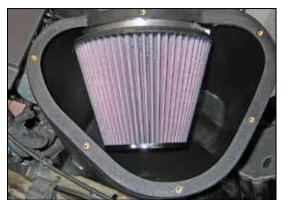
29. Install the K&N<sup>®</sup> air filter onto the filter adapter and secure with the provided hose clamp. NOTE: Drycharger<sup>®</sup> air filter wrap; part # RF-1036DK is available to purchase separately. To learn more about Drycharger<sup>®</sup> filter wraps or look up color availability please visit http://www.knfilters.com<sup>®</sup>.
