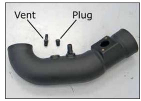
21. On vehicles that have an EVAP vent line attached to the intake tube, install the 3/8" vent fitting into the K&N<sup>®</sup> intake tube. On vehicles that do not have the EVAP vent line attached to the intake tube, install the NPT plug into the intake tube. **NOTE: Plastic NPT fittings are easy to cross thread. Install the vent fitting "hand" tight, then turn it two complete turns with a wrench.**
