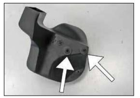
16. Install the airbox mounting grommets onto the two mounting studs installed on the K&N<sup>®</sup> airbox.
