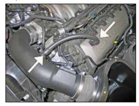
27. Install the crankcase vent hose to the fitting on the K&N<sup>®</sup> intake tube and onto the valve cover. Vehicles equipped with an EVAP vent line, connect it to the fitting installed in the K&N<sup>®</sup> intake tube.
