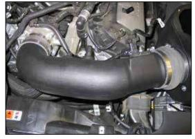
26. Install the K&N<sup>®</sup> intake tube into the silicone hose at the airbox and then into the silicone hose at the throttle body; secure with the provided hose clamps.
