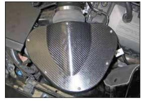
30. Install the K&N<sup>®</sup> airbox lid and secure with the provided hardware.
