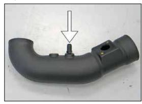
20. Install the crankcase vent fitting into the  $K\&N^{\circledast}$  intake tube as shown.
