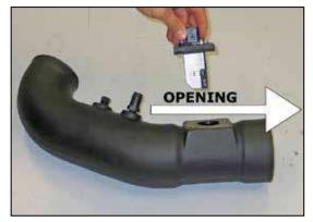
25. Install the mass air sensor assembly into intake tube and secure with the provided hardware. NOTE: Be sure the open end of the sensor is facing the filter end of the tube.
