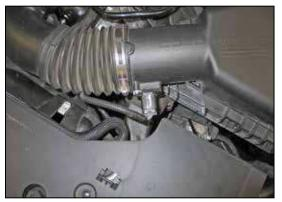
6. Unhook the mass air sensor electrical connection.
