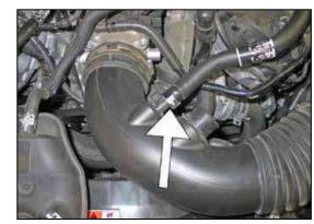
7. Disconnect the crankcase vent hose from the factory intake tube and valve cover port and remove the vent tube from the vehicle. **NOTE: Some models may be equipped with the EVAP vent hose, it will be necessary to disconnect the EVAP vent hose from the factory intake tube.**
