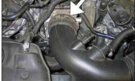
8. Loosen the hose clamp that secures the factory intake tube to the throttle body.
