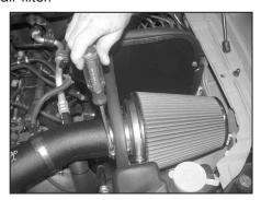
30. Install the K&N $^{\otimes}$  air filter assembly onto the K&N $^{\otimes}$  intake tube as shown; secure with the provided hose clamp.
