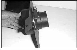
10. Assemble the mass air sensor, heat shield and adapter using the gasket and hardware provided.
