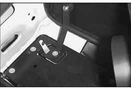
21. Secure the bracket to the airbox mounting tray using the bolt removed in step 19.
