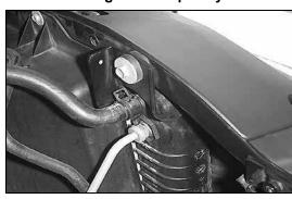
16. Measure over and down  $\frac{1}{2}$ " on the radiator mounting bracket and mark.
