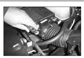
3. Loosen the hose clamp on the intake hose at the
