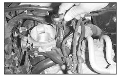
12. Remove the nut that retains the throttle cable bracket. **NOTE: The nut will not be reused.**
