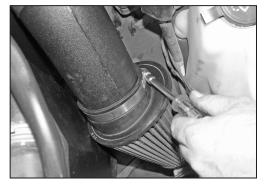
40. Install the air filter element onto the intake tube rotate, for best clearance and secure it with the provided hose clamp.
