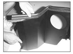
20. Install the 5/8" OD grommet and a flat washer over the original air box mounting stud.
