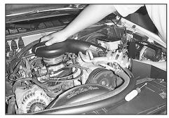
32. Install the primary intake tube onto the adapter and tighten the second midi hose clamp.
