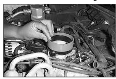
19. Install the 4"ID silicone hose over the adapter and tighten using a provided midi clamp.
