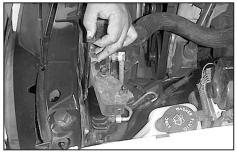
9. Pull the release tab and slide the retainer bracket upward to remove it from the radiator core support.
