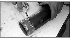
29. Using the hose clamp provided, attach the silicone step hose onto the end of the primary intake tube.
