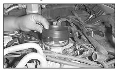
16. Install the adapter and hand tighten the three 6mm allen bolts.
