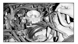
13. Install the short coupling nut onto the throttle body stud mentioned in the previous step.
