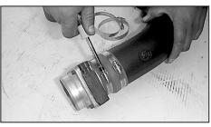
30. Using the hose clamp provided, attach the silicone step hose to the mass air sensor with the directional arrow as shown above.
