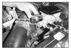
2. Disconnect the mass air sensor and air temp. sensor electrical connections.
