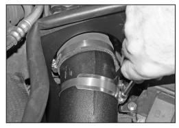
39. Attach the saddle/bracket assembly to the secondary intake tube using the provided hose clamp.
