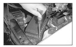
5. Loosen the four screws that retain the air box top to the air box base.
