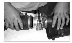
25. Remove the mass air sensor from the stock intake tube and air box top.
