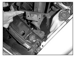
8. Pull the air box upward firmly to release the grommets from the retainer bracket.
