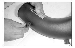
28. Install the air temp. sensor into the grommet.
