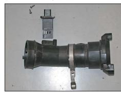
19. Remove the mass air sensor from the factory mass air sensor housing using the Torx wrench provided.
