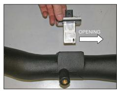
22. Install the mass air sensor assembly into the K&N® intake tube.
