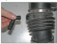
16. Remove the crank case vent fitting from the factory intake tube as shown.
