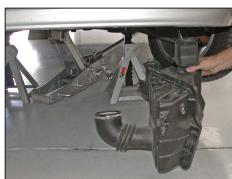
14. Lower and remove the air box assembly from the vehicle.
