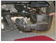
12. On vehicles equipped with an air box cover, lower the cover and remove it from the vehicle.
