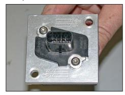
21. Using the factory mass air bolts, install the mass air sensor into the K&N® mass air adapter as shown.
