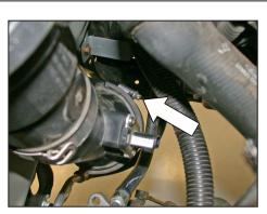
7. Loosen the hose clamp, which secures the mass air sensor housing to the lower intake housing.
