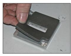
20. Apply the provided gasket onto the K&N® mass air adapter as shown.
