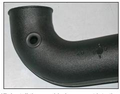
17. Install the provided grommet into the  $K\&N^{\circledast}$  intake tube as shown.
