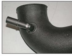
18. Install the crank case vent fitting removed in step #16 into the grommet installed into the K&N® intake tube in step #17 as shown.
