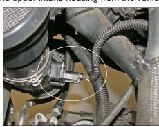
6. Depress the locking tab on the mass air sensor electrical connection and then disconnect the electrical connection.
