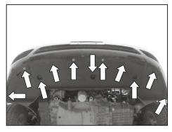
10a. On vehicle's equipped with the splash shield, remove the six bolts and five plastic screws which secure the splash shield to the bumper cover, then remove the splash shield from the vehicle.
