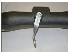
24. Install the provided bracket (010063) onto the K&N® intake tube with the provided hardware as shown.
