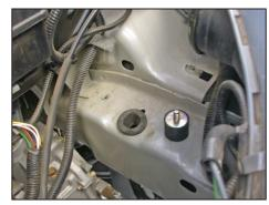
25. Install the rubber mounted stud into the threaded hole in the frame rail as shown.
