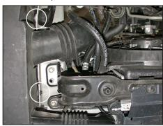
11. On vehicle's equipped with an air box cover, remove the two bolts which secure the cover to the frame rail, and the bolt which secures the intake snorkel to the radiator core support.
