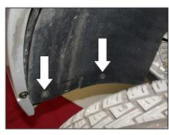
10. After jacking up the car and placing on suitable jack stands and chocking the rear wheels, remove the two bolts which secure the air box on equipped vehicle's or the one bolt on splash shield equipped vehicle's to the inner finder well.
