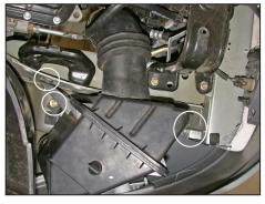
13. Remove the three bolts which secure the lower air box to the inner fender well.
