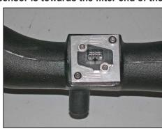
23. Secure the mass air sensor assembly into the  $K\&N^{@}$  intake with the provided hardware as shown.
