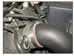
27. Reconnect the crank case vent hose to the fitting installed into the K&N® intake tube in step #18.
