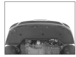
30a. On vehicle's that were equipped with the splash shield, reinstall with the bolts removed in step #10a.
