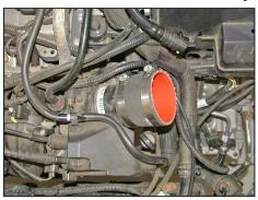
15. Install the silicone hose (08192) onto the throttle body and secure with the provided hose clamp.
