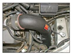
26. Install the K&N® intake tube assembly into the silicone hose at the throttle body and onto the rubber mounted stud, then secure with the provided hardware.
