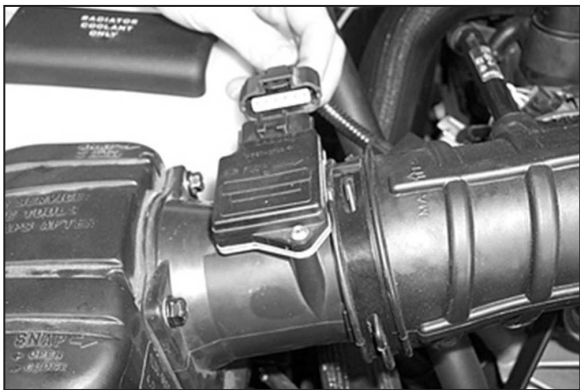
2. Disconnect the mass air sensor electrical connection.
