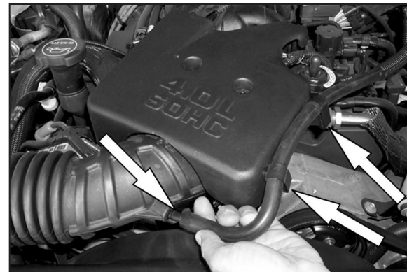
5. On vehicles that come with a second vent line, remove hose from intake tube then release the two clips that retain the hose to the engine cover.
