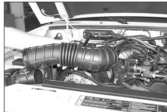
6. Loosen the hose clamp at the throttle body and at the mass air sensor, then remove the stock air intake tube as shown.
