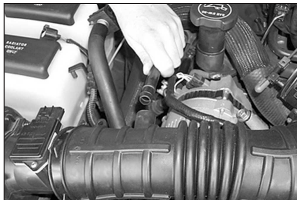
4. Remove the crankcase vent hose from the stock intake tube as shown.
