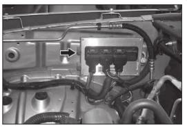
7a. On 2008 and later model vehicles, remove the ECU mounting bolt shown.
