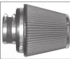
26. Install silicone hose (#08630) onto the air filter adapter and secure with the provided hose clamp.
