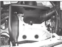
23. Install the heat shield into the engine compartment. Align the bottom rear mounting bracket with the threaded stud on the lower inner fender. Align the upper rear mounting bracket with the ECU mounting stud. Secure with the factory ECU mounting nut and provided hardware.
