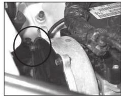
8. Remove the timing cover bolt (shown).
