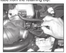
3. Release the red locking tab, then disconnect the air temperature sensor electrical connection.
